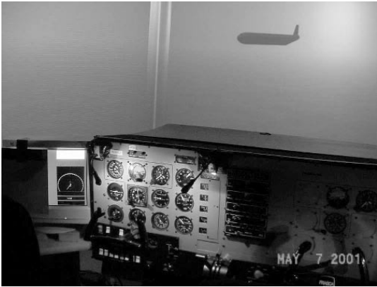
Figure 1. Frasca instruments, data link and CDTI displays, and traffic close-up. The CDTI is shown on the black display to the left of the instrument panel; the data link message appears in the white rectangle just above that.
