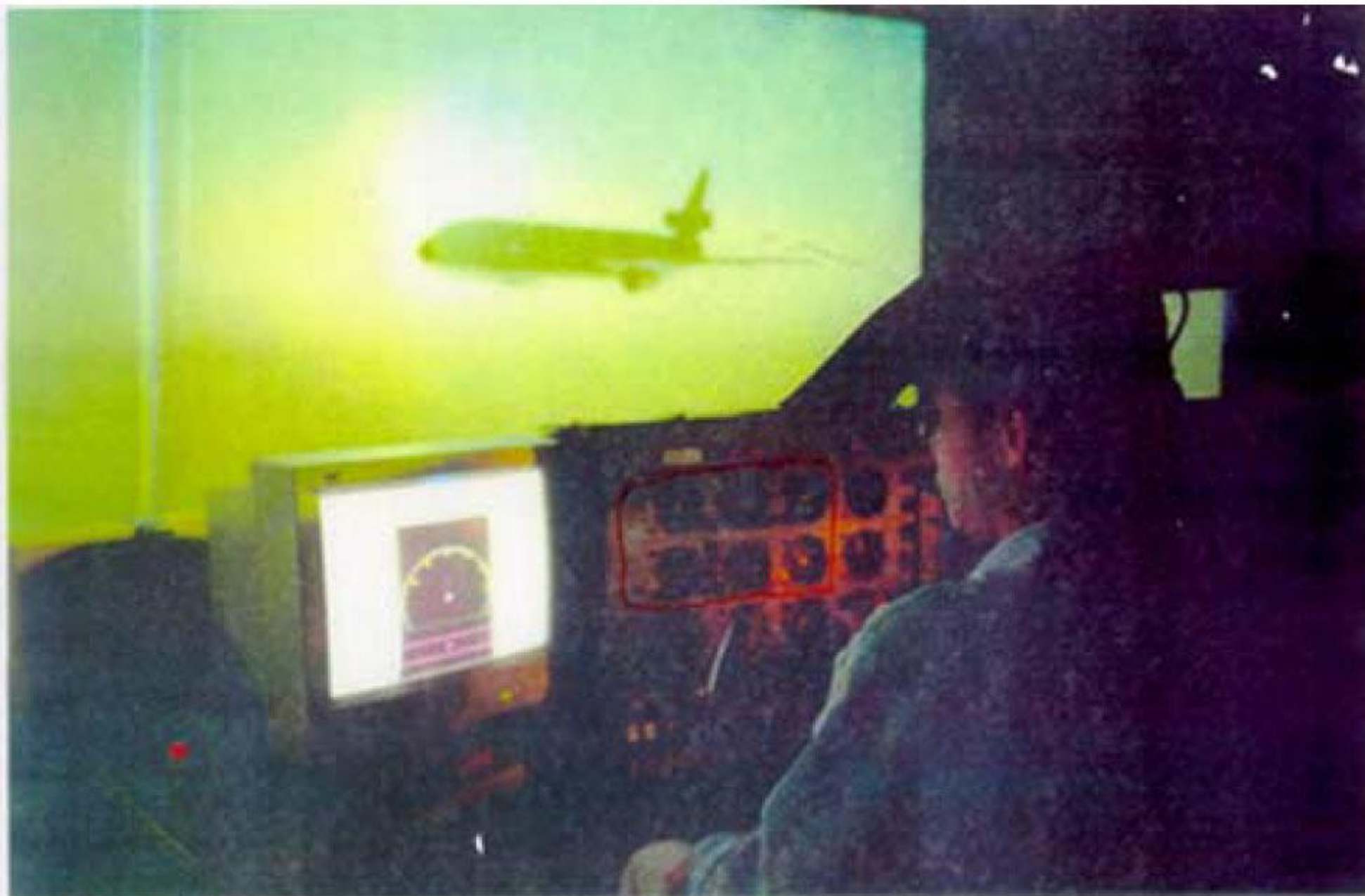
Figure 3. The simulation environment, showing the CDTI to the left and the instrument panel (IP) to the right.
