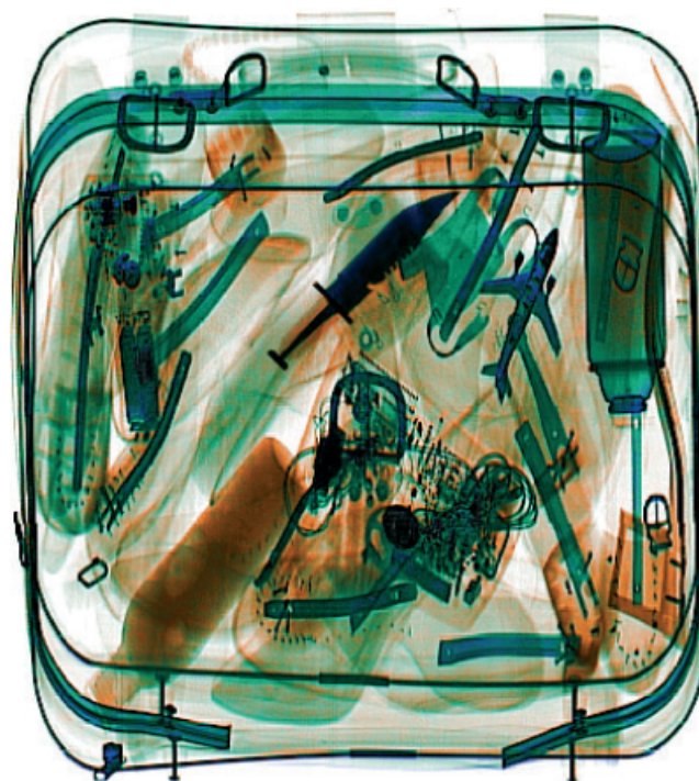
Fig. 1. Example of a target-present stimulus image. The target (the blade and shaft show up in dark blue, and the handle in orange) is a little above the center of the image, to the left of the toy airplane.
