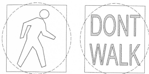
Figure 4—Illustration of how different signals fill the meter aperture.
