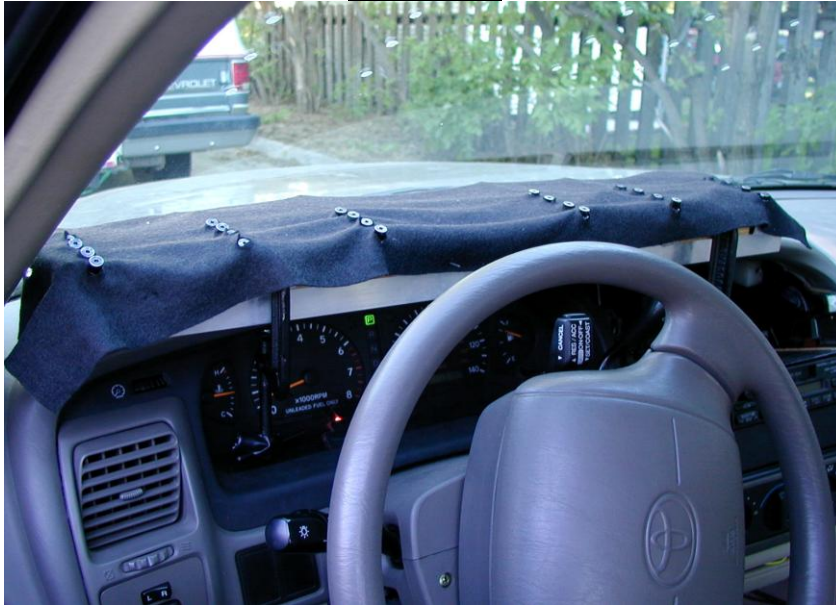
Laser projection unit affixed to the dashboard of Avalon test car.
