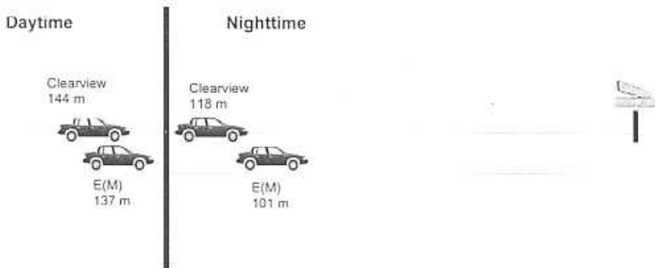
Figure 8. Reading distance of Clearview versus Standard Highway font.
